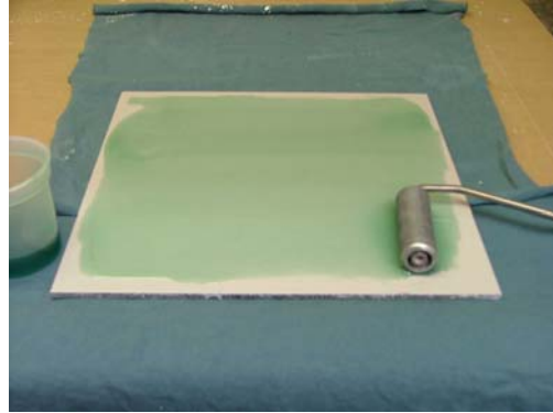
Wetting out back of gelcoat with resin
