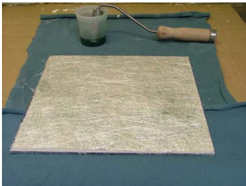
Apply precut glass into wet resin
