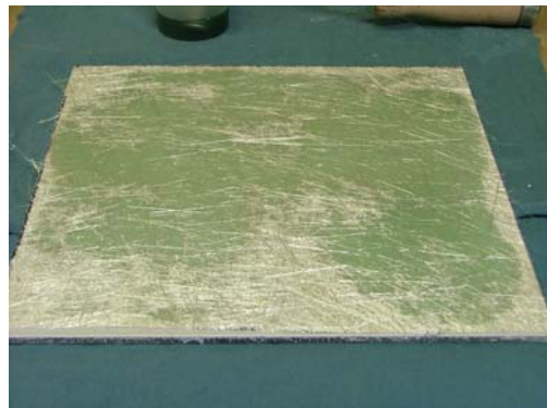
Resin soaking up through glass
